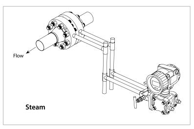
**Note:** For steam or other elevated temperature services, it is important that temperatures at the process connection do not exceed the transmitters process temperature limits.
