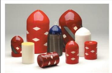
Girard Polly-Pigs, constructed of open cell polyurethane foam, are available in light, medium and heavy densities. They are designed to negotiate pipeline configurations that other pigs cannot, such as "tees," elbows and multiple diameter changes.
