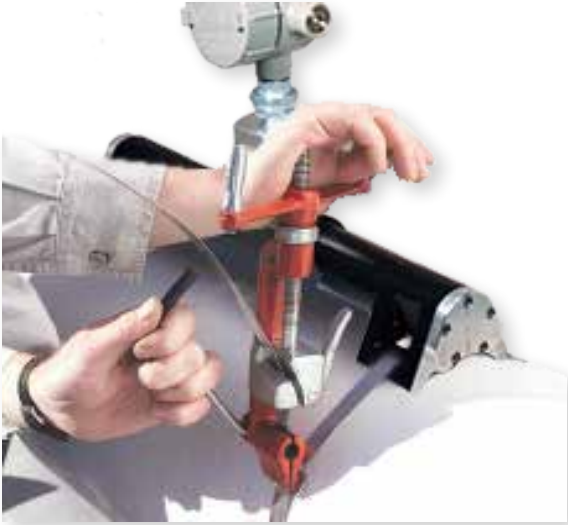
Banding tool for securing CD52 Bandit and 316-SS to pipeline
